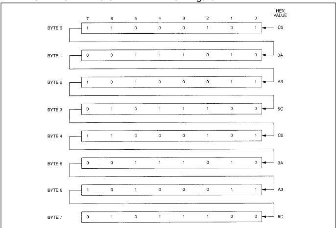
**NOTE:** THE PATTERN RECOGNITION IN HEX IS C5, 3A, A3, 5C, C5, 3A, A3, 5C. THE ODDS OF THIS PATTERN BEING ACCIDENTALLY DUPLICATED AND CAUSING INADVERTENT ENTRY TO THE PHANTOM CLOCK IS LESS THAN 1 IN 10<sup>19</sup>. THIS PATTERN IS SENT TO THE PHANTOM CLOCK LSB TO MSB.
